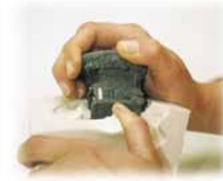
The mould is carefully stripped from the master
