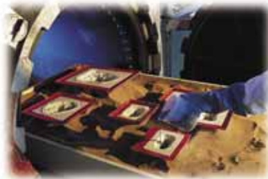
Filling master moulds with resin
