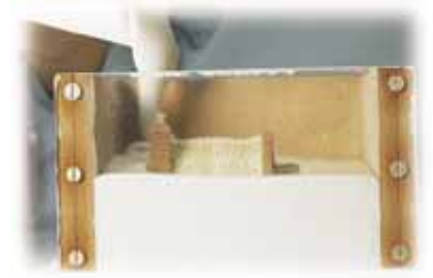
Wax in silicone to create first block mould
